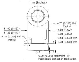
0.13 (0.005) Minimum Ref. (applies to top edge of gasket or edge of crimp, whichever is higher)
